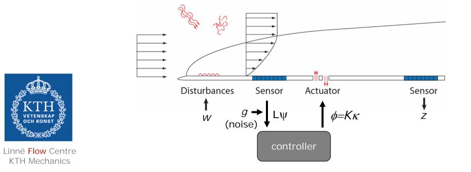
Find an optimal control signal  $\phi(t)$  based on the measurements  $\psi(t)$  such that in the presence of external disturbances w(t) and measurement noise g(t) the output z(t) is minimized.
